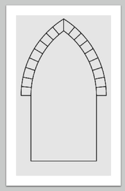
• **Pointed arches**: Curved masonry construction that spans an opening such as a portal or window. Pointed arches were a feature of the Gothic era, that evolved from the round Romanesque arches.
